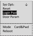
**Reset:** The device can be restored into factory defaults or default settings.
